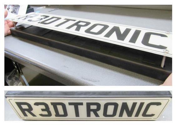
6 Mark the centre between the number plate fastening holes on the vehicle body
