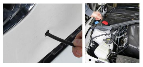
9 Place the Stealth Plate up to the vehicle body and using a spirit level to ensure that the plate is level, mark the vehicle body through the x4 Stealth Plate fixing holes with a bradawl or screwdriver
