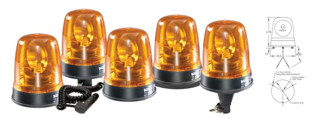
Tough polycarbonate impact resistant amber lens, Durable black ABS base • Quiet belt driven reflector rotates around fixed H1 globe (not included) Dual voltage motor 12V or 24V, change bulb to suit voltage, RFI suppressed • 4.6 Amp draw at 12V (based on 55W globe), Flash rate nominal 160
